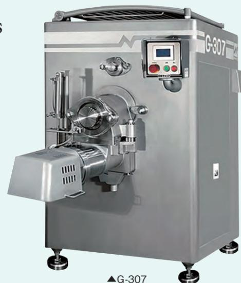
G-307 and G-407 multi-stage grinders are equipped with pre-setters standard. Bone collectors optional. (2 patents registered, 1 pending)
