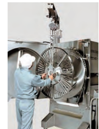
Detaching the disk and impeller knife
