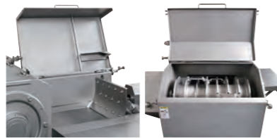
Top/front cover equipped with safety devices
