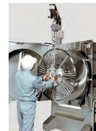
Detaching the disk and impeller knife
